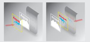
The SurePress L-4733A/AW provides the flexibility of printing white first or last
